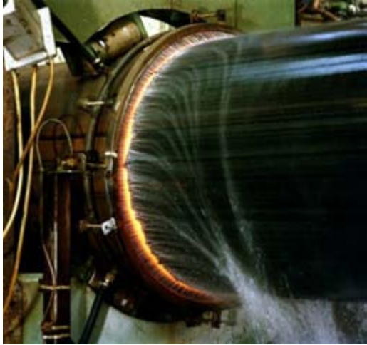
Figure 15: Detailed view on induction coil and heated zone during bending
