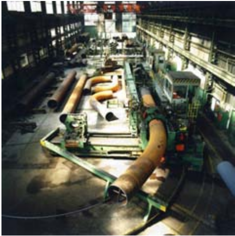
Figure 14: Hot induction bending of 48" line pipe at Mannesmann Bending Plant
