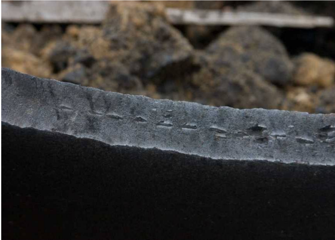
Figure 19: Fracture surface of arrest pipe
